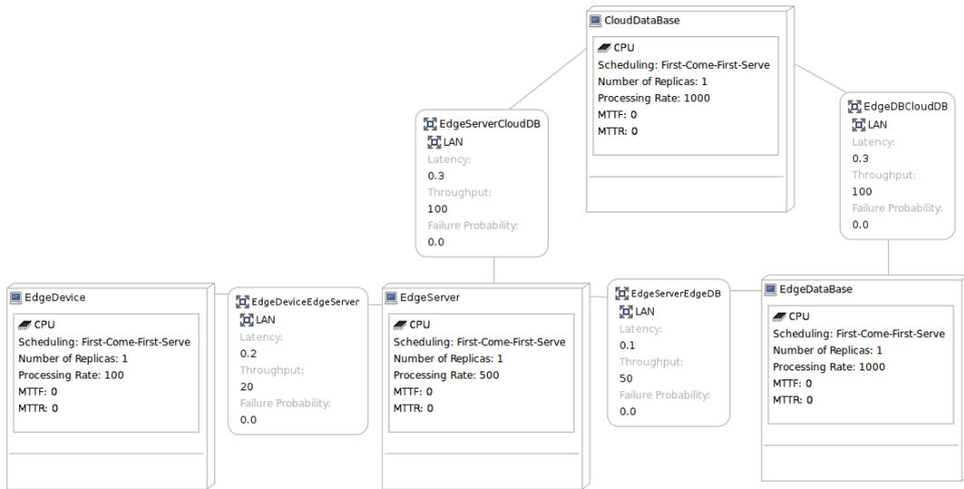
FIGURE 7.20: IoT Palladio Resource Environment 2 DB
