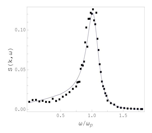
Figure 1.5 – The OCP normalized dynamic structure factor in comparison with the simulation data of [9] (boxes) at  $\Gamma$  = 8 and q = 1.389.
