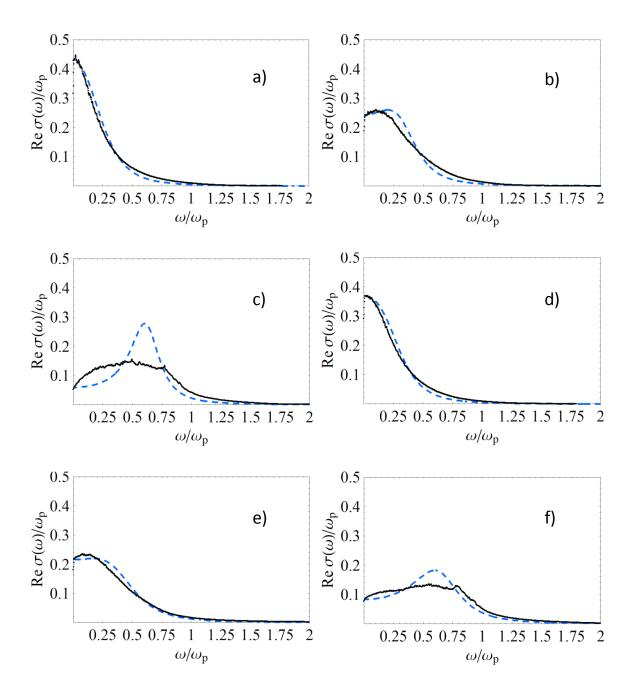
Figure 3.2 Real part of the internal dynamic conductivity for aluminum plasmas as simulated in Ref. [51]: (a) 10 kK, 1.4 g  $\cdot$  cm<sup>-3</sup>; (b) 10 kK, 1.0 g  $\cdot$  cm<sup>-3</sup>; (c) 10 kK, 0.5 g  $\cdot$  cm<sup>-3</sup>; (d) 25 kK, 1.4 g  $\cdot$  cm<sup>-3</sup>; (e) 25 kK, 1.0 g  $\cdot$  cm<sup>-3</sup>; (f) 25 kK, 0.5 g  $\cdot$  cm<sup>-3</sup>.
