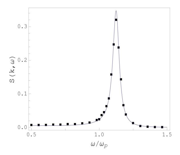
Figure 1.1 – The OCP normalized dynamic structure factor in comparison with the simulation data of [9] (boxes) at  $\Gamma$  = 0.993 and q = 0.6187.
