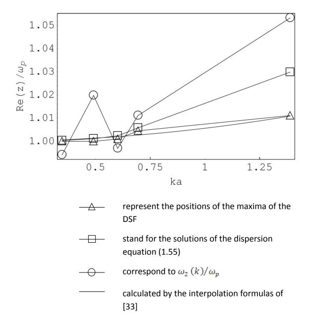
Figure 1.10 – The plasmon dispersion relation, i.e., the real part of the solution of the dispersion equation (1.55) vs. ka at  $\Gamma$  = 8.
