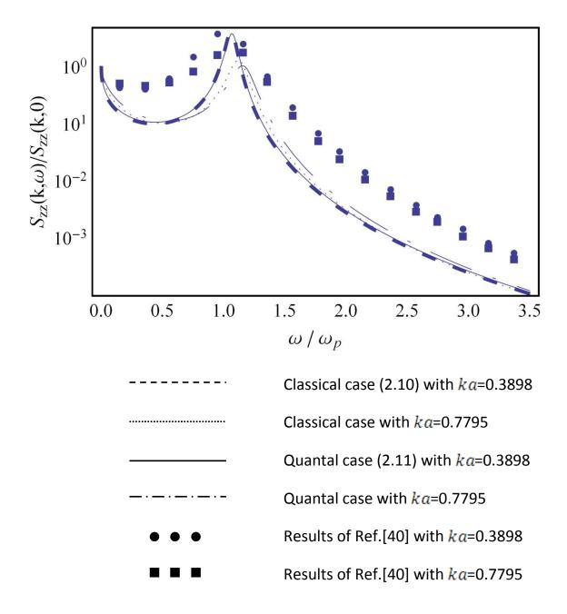
Figure 2.4 – Normalized charge-charge dynamic structure factor vs. frequency at  $\Gamma$  = 2 and  $\lambda_{ep}$  = 0.4.
