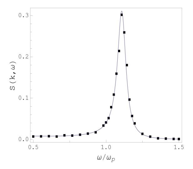
Figure 1.2 – The OCP normalized dynamic structure factor in comparison with the simulation data of [9] (boxes) at  $\Gamma$  = 1 and q = 0.49109.
