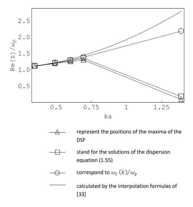
Figure 1.6 – The plasmon dispersion relation, i.e., the real part of the solution of the dispersion equation (1.55) vs. ka at  $\Gamma$  = 0.993.
