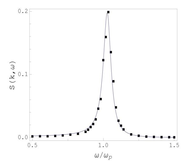
Figure 1.4 – The OCP normalized dynamic structure factor in comparison with the simulation data of [9] (boxes) at  $\Gamma$  = 4 and q = 0.6945.
