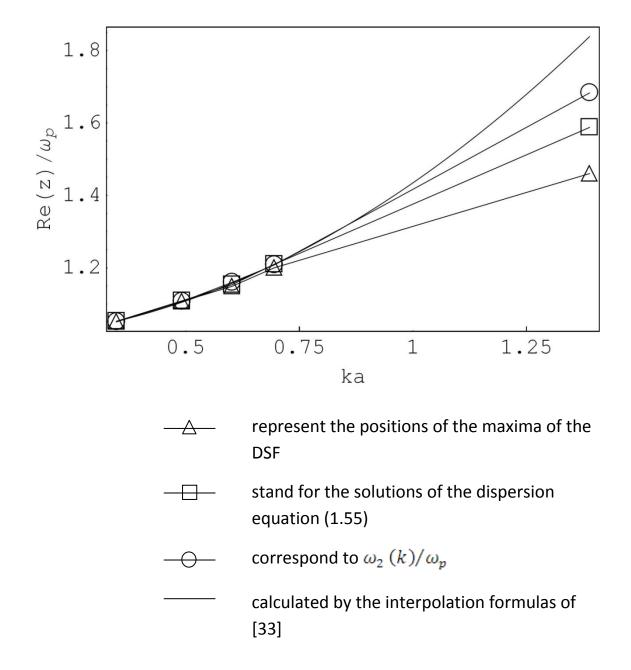
Figure 1.7 – The plasmon dispersion relation, i.e., the real part of the solution of the dispersion equation (1.55) vs. ka at  $\Gamma = 1$ .
