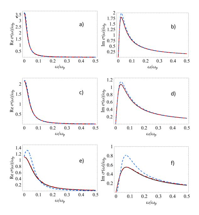
Figure 3.1 Real and imaginary parts of the internal dynamic conductivity for a TCP at the thermodynamic conditions simulated in [11]: (a) and (b)  $\Gamma$  =0.5,  $r_s$ =0.4; (c) and (d)  $\Gamma$  =0.5,  $r_s$ =1; (e) and (f)  $\Gamma$  =2,  $r_s$ =1. Three different models are used for  $\sigma$ : Drude-Lorentz formula (3.43) (solid line), two-moment model (3.23) with q given by (3.35) (dashed line), and its static value (dash-dot). The relevant parameters are taken from Table 1.
