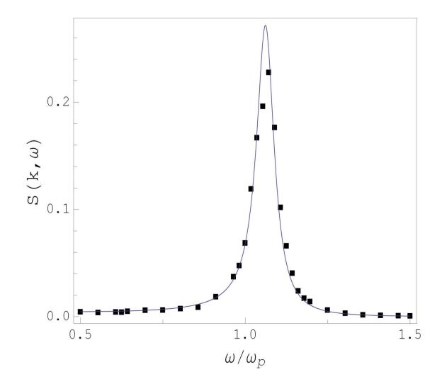
Figure 1.3 – The OCP normalized dynamic structure factor in comparison with the simulation data of [9] (boxes) at  $\Gamma$  = 2 and q = 0.60145.
