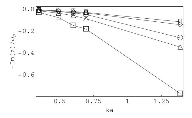
Figure 1.11 – The plasmon mode damping decrement, i.e., the imaginary part of the solution of the dispersion equation (1.55) vs. ka for  $\Gamma$  = 0.5 (squares),  $\Gamma$  = 1.0 (triangles),  $\Gamma$  = 2.0 (circles),  $\Gamma$  = 4.0 (diamonds), and  $\Gamma$  = 8.0 (rectangles).
