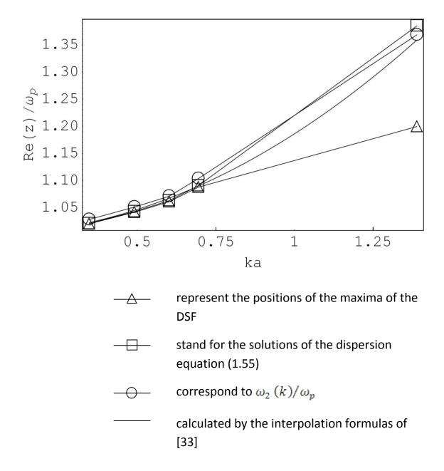
Figure 1.8 – The plasmon dispersion relation, i.e., the real part of the solution of the dispersion equation (1.55) vs. ka at  $\Gamma$  = 2.
