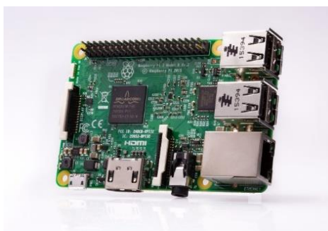
Figura 1. Tarjeta Raspberry Pi 3 modelo B ( https://www.raspberrypi.org/ )
