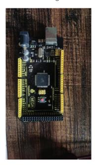
Figura 3. Tarjeta Arduino MEGA.
