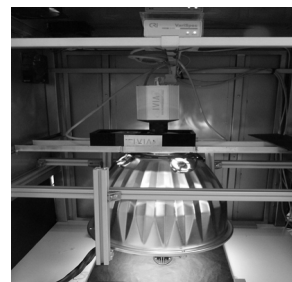
Figure 2. Hyperspectral camera CoolSnap ES structure and LCTF filters. Source: The Authors.
