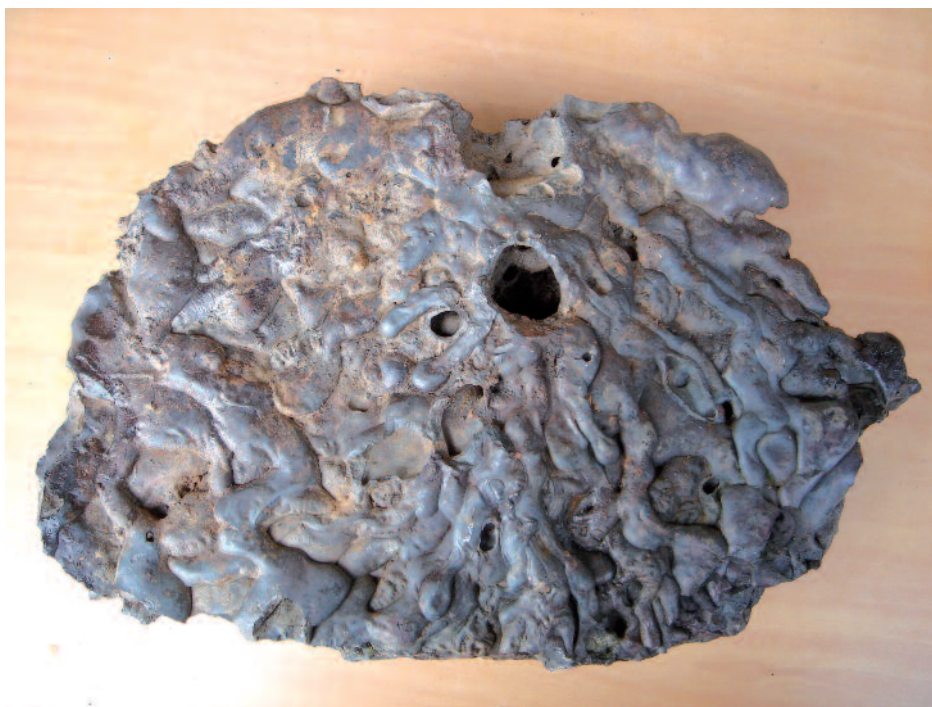
Figure 12. Large slag (36 cm) collected in a deposit located less than 1 km from the furnace of Azarola in Galdakao (Bizkaia).
