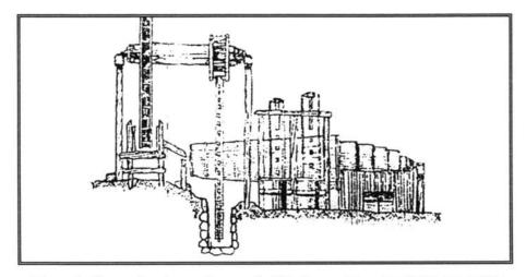
Figure 2.- The machine for washing ores built by the magister naturalis Munteanu Urs
