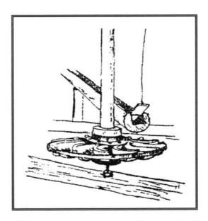
Figure 7.- The water admission system of the horizontal wheel [8]
