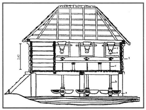
Figure 4.- Section through the mill: a. water-wheel, b. wooden shaft, c. iron shaft, d. socle of the mill-stones, e. feeder, f. loading funnel [8]
