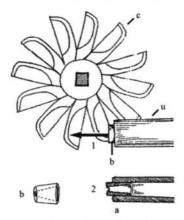
Figure 5.- The popular wooden turbine: a wheel equipped with «spoons» installed in a Mill.
