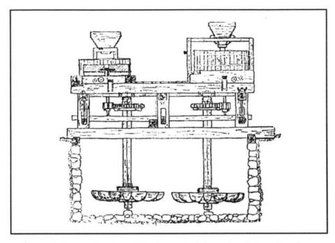
Figure 8.- Water mill with two dip buckets and belt drive – Râu de Mori, Hunedoara County [8]
