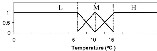
Figure 7 A group of possible fuzzy sets defining the output variable “temperature”
