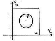
To symplify, we take T of area equal to 1.— We suppose  $\omega$  and T periodically reproduced throughout the plane  $(y_1,y_2)$  Anyway, T,  $\omega$  . Will denote both the hole and rectangle of the figure and all the others obtained via periodic translations.
